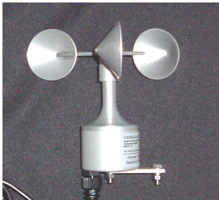
Figure 2.2: three cups wind speed sensor.
